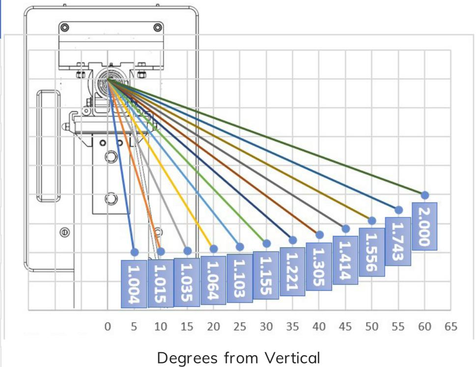
The cable may be 5° from vertical when the lift is fully lowered but depending on the geometry of the installation, the cables may be at 35° from vertical when the lift is fully raised. The tension will increase from 1.004 times the straight-line vertical tension to 1.221 times (22.1%).
