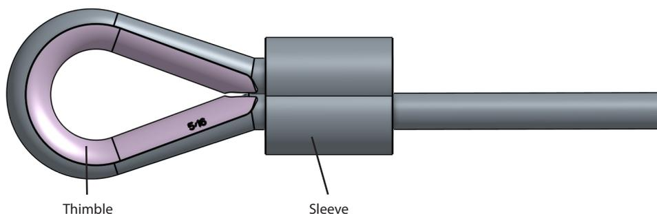
BH-USA recommends only using zinc-coated copper sleeves for use in marine environments or sudden catastrophic failure can occur.
