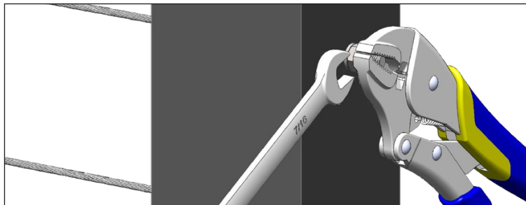
Figure L. Option one (1) is to hold the back of the stud with vice grips while tightening the nut.
