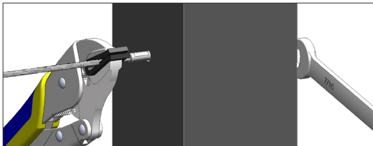
Figure M. Option two (2) is to use a cable grip pad to hold the cable just outside the post while tightening the nut.
