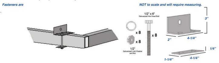
**Wood Bunk Installation** - Place the two carpeted wood bunks (included) in place alon side the brackets so that the angle is on the inside. Mark these points, drill a hole large enough to slide the 1/2" bolt through, this will secure the bunks to the brackets.
