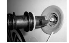
Inflate the tube to approximately 80-90% full (approx. 4 minutes.) The tube will be erect but very soft at this stage. Do not inflate fully until after the springs are attached.
