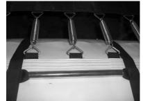
IMPORTANT: Properly mounted, the ladder straps should run parallel to each other around the tube with three springs and  $\Delta$ -rings between the ladder straps as shown.
